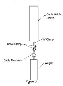
With cable weights 3" off the floor and the cables hanging straight, use Draper supplied snap links to attach netting to cables. Snap links should be placed approximately 24" on center and should capture at least two or three stands of the netting material. The first snap link should be placed about 2" above the cable weight.
